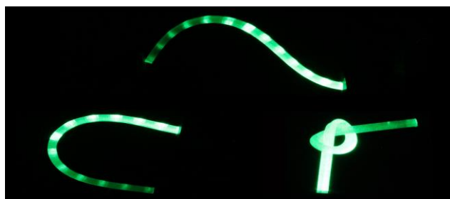
3D-printed, flexible, light-conducting waveguides
